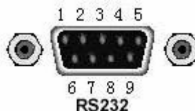
Figure 5-3 Rear Panel RS232 Interface
